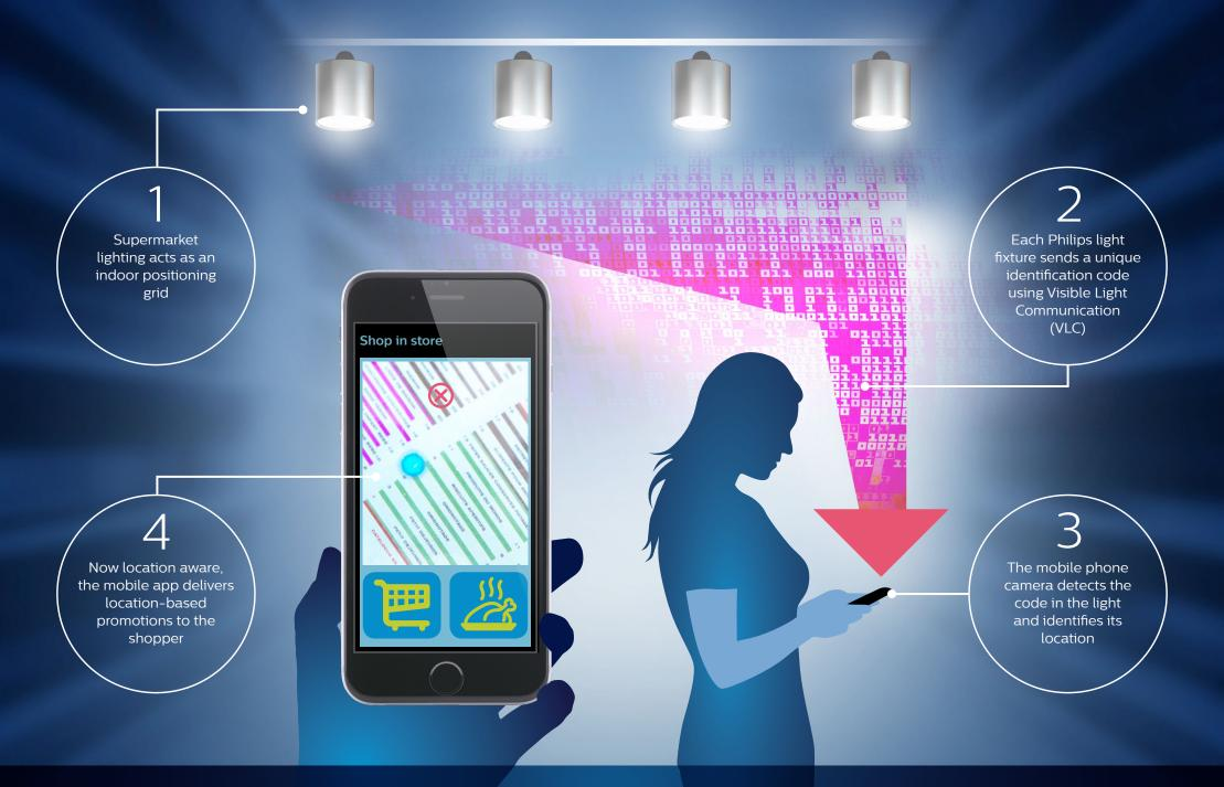
**Philips LED-based indoor positioning technology** is easy to scale, accurate to a sub-meter, does not require additional investments besides the light fixtures themselves, and offers at least 50% energy savings.
