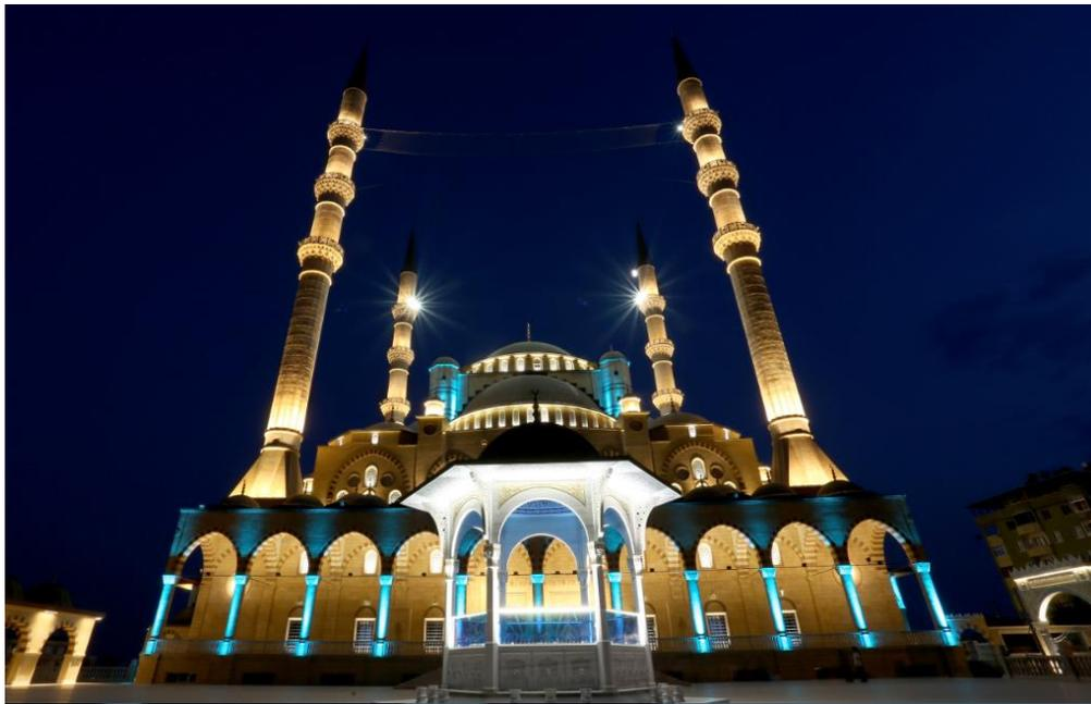
For the new illumination of the mosque, a mix of colored and warm white LED lighting is used. For the exterior, the columns of the mosque are illuminated with [Philips Vaya Flood LP RGB](#) luminaires, while warm white light is used in the back hall to accentuate wall illustrations.
