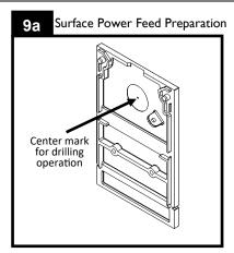
For surface junction box installation, power feed to fixture module is done through the endcap. Use masking tape on all outside surfaces, turn over and place on a wood block. Align with center mark as shown and drill a 7/8" diameter hole.
