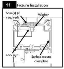
From below fixture secure 1/4" ID washer and 1/4"-20 hex nut to ceiling bracket 1/4"-20 stud. If ceiling is not level, install supplied shims as required then tighten 1/4"-20 hex nuts.
