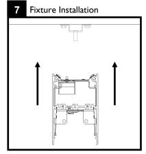
Raise module 1 towards ceiling, supporting both ends a few inches below ceiling level.
