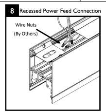
While supporting the module in the air complete power entry wiring connections. Ensure all connections are secure and all wires are neatly tucked inside fixture wiring cavity.
