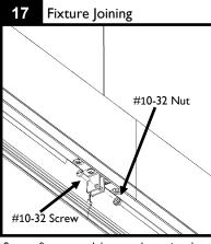
Secure fixture modules together using the two #10-32 machine screws and the two #10-32 nuts supplied. Tighten until joint seam is tight. **Note: Do not overtighten.**
