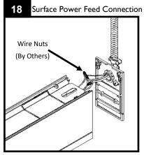
For surface mounted junction box, connect conduit and required connectors (by others) to drilled endcap.
