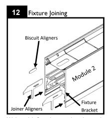
With module 2 on the ground, tap biscuit aligners inside top screw chase. Ensure biscuit aligners are inserted more than half way inside fixture housing. Insert joiner aligners inside lower screw chase as shown. Ensure orientation is correct for locking tab to engage and lock inside fixture bracket.
