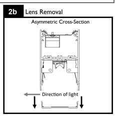
Remove lens from fixture and set aside until fixture installation is complete. Use cotton gloves to handle lenses and keep in a clean environment. **Note:** Do not mix symmetric fixture lenses with asymmetric fixture types as they are different.
