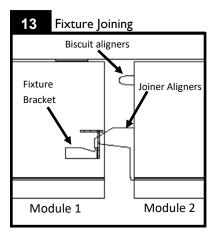
Bring modules together and engage joiner aligners in module 2 on fixture bracket in module 1. Note: Do not secure module 2 to the ceiling at this step.
