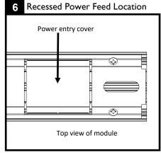
Determine fixture power feed method and location. For a recessed utility box installation, break off power cover tabs using a flat screwdriver at required end only.
