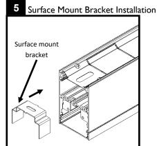
Insert surface mount brackets approximately 2 inches inside module 1. Ensure bracket engages and slides inside upper fixture module channel. Ensure slot in fixture reflector aligns with slot in surface mount bracket.
