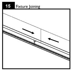
Ensure all connections are secure and all wires are neatly tucked inside fixture wiring cavity. Slide fixture modules together gently. With module 1 and module 2 butted together, secure the non joining end of module 2 to the ceiling.
