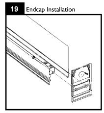
Slide endcap onto end of fixture module and secure from below using two #8-32 X 5/16" screws. Tighten screws until endcap seam is tight. **Note: Do not overtighten.**
