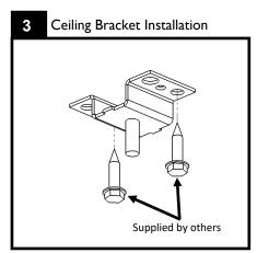
Determine location of ceiling brackets. Use table on page 1 for exact dimensions. Center and install ceiling brackets to structure (studs or cross-braces) using appropriate hardware (by others)
