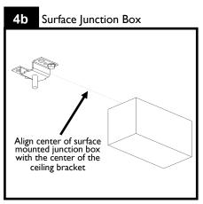
For a surface mounted junction box, install junction box as required. For a cleaner install and better alignment with installed fixture modules, center junction box and conduit exit with center line of ceiling brackets.
