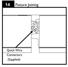
With module 2 supported complete wiring connection using provided quick wire connectors.
