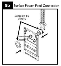
Prepare power feed by installing the conduit and the connectors (by others) to the drilled endcap. Refer to steps 13 and 14 for power connections and endcap installation.
