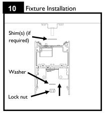
Raise module 1 to ceiling, align ceiling bracket 1/4"-20 stud with housing slot and surface bracket slot.
