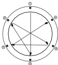
Use several rotations of the following sequence to firmly tighten the lens ring screws, to 25 in/lbs.
