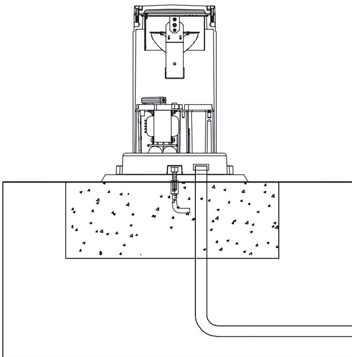
1. Prepare the site with adequate excavation and install the anchor bolts and 3/8" couplers per factory supplied template <sup>1</sup>.
