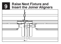
Raise next fixture to ceiling and insert the joiner aligners into the corresponding slots on the already installed fixture.
