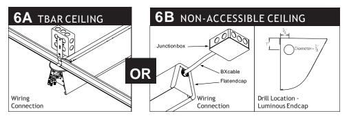
For non-accessible ceilings, drill 7/8 hole (location marked on Flat endcap: see diagram on right for drill location on Luminous endcap). Attach armored cable from the junction box (supplied by others) according to code.
