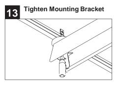
Tighten mounting bracket. Reinstall socket saddles or LED modules (remember to reconnect the low voltage wire harness). Install power plate and plug.
