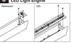
Remove socket saddle or LED light engine to gain access to mounting channel. When removing LED light engine be sure to disconnect the low voltage wire
