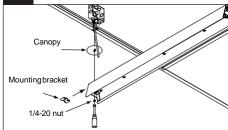
Remove socket saddle or LED light engine to gain access to mounting channel. When removing LED light engine be sure to disconnect the low voltage wire harness.
