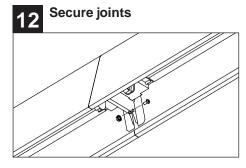
Join fixtures using supplied #8 screws and lock-nuts.
