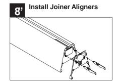
On the floor, slide variable mount bracket into next fixture in run. Attach joineraligner brackets, power plate and plug into opposite side.
