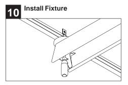
Using the supplied 1/4-20 nuts attach the fixture to the ceiling through the slots in the top of the fixture. DO NOT FULLY TIGHTEN. The mount should be able to slide, but be snug.
