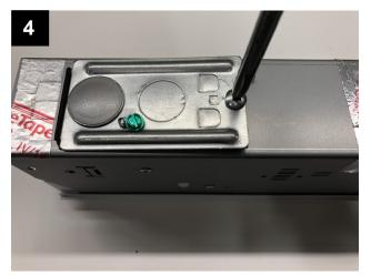
Align wire cover mounting hole with hole in housing.
