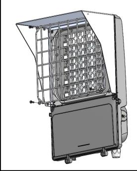
Note: Wireguard can be mounted over Visor or Glare Shield. When nesting wireguard and Visor or Glare Shield together use the longer 5/8" screws that are provided with the Wireguard.
