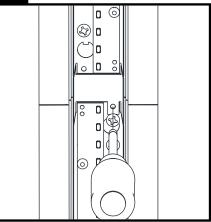
Mount the LED pan connector with the supplied screw in the joiner kit. Note: this step is not required for louvers.
