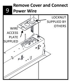
At power location(s), feed power wires through supplied wire access plate. Complete all wiring connections using wire nuts supplied by others.
