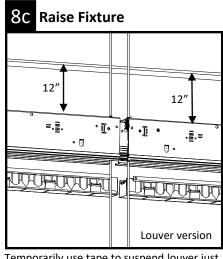
Temporarily use tape to suspend louver just below fixture. <u>DO NOT ALLOW LOUVER TO</u> HANG FROM ELECTRICAL WIRES.
