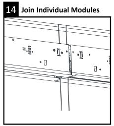
Gently slide housing modules together, ensuring joiner aligners are engaged inside the trim in the adjacent module.
