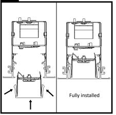
Install louvers previously removed for installation.
