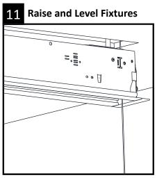
Once the power connections are complete, pull the aircraft cable to raise all modules to just below the ceiling.
