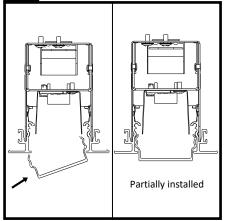
Installation Tip: For easier installation, start at a housing end or a joint by placing lens at an angle and squeezing opposite end in slightly from the other side to insert inside housing.
