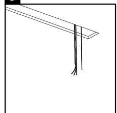
Install drywall ceiling and cut required opening as shown in **figure A** on page 2 or **figure B** on page 3.
