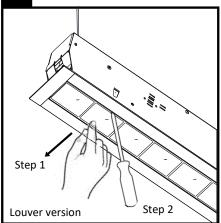
To remove louver, first push louver edge away with one hand, then gently pry opposite side with a thin, flat screwdriver.
