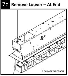
Temporarily use tape to suspend louver just below fixture. <u>DO NOT ALLOW LOUVER TO</u> <u>HANG FROM ELECTRICAL WIRES.</u>
