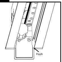
Push up drop lens endcap flush to bottom of trim while hand tightening with supplied screws.(8-18 x 3/8 Pan)
