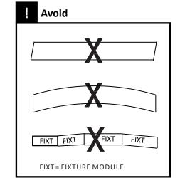
The straightness and accuracy of the cut-out in the drywall is crucial in ensuring proper fit for the fixture.
