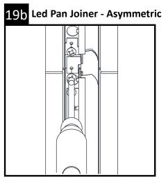
Mount the LED pan connector with the supplied screw in the joiner kit. There are two pieces for the asymmetric fixture.
