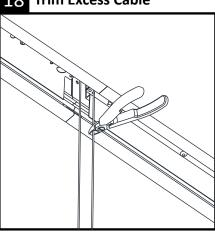
Trim suspension cable approximately 9 inches below the ceiling level. Tuck all excess cable inside the upper wiring cavity.
