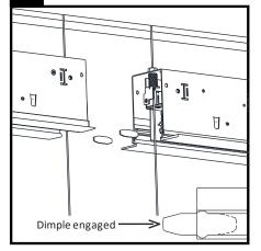
At joint location(s), gently tap provided joiner aligners inside one module only. Two joiner aligners are required for each joint. Important: To insert aligners, tap gently with a hammer until half is inserted into the joiner channel. Be sure to engage the dimple as shown.
