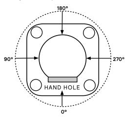
For Factory Installed Options and Accessories, Specify Orientation from Hand Hole and Height Above Pole Base Where Required.
