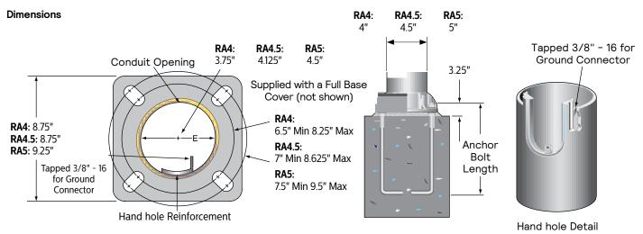
NOTE: Factory supplied template must be used when setting anchor bolts. Gardco will not honor any claim for incorrect anchorage placement from failure to use factory supplied templates.
