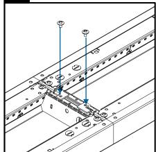
Once locking plate is inserted, secure locking plate to the crossplate. Using a head screwdriver, tightened screws until the two fixtures pull together creating a seamless gap.
