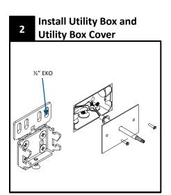
Determine power feed location, install 2"x4" utility box (supplied by others) parallel to fixture. Utility box must be installed at least 3.8" from end of fixture. Bottom of utility box must not be lower than the bottom of fixture. Complete connections at box with supplied power cord. Attach cover bracket. Punch power access hole in cover, feed power cord through, attach strain relief and box cover.
