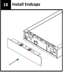
Place endcap on top of crossplate. Align to luminaire
