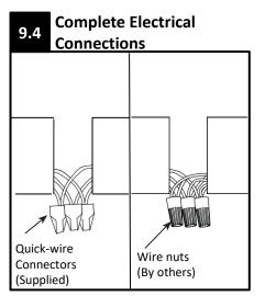
Complete in-row electrical connections. NON-POWER LOCATIONS: Use supplied quick-wire connectors. Tuck wires into wire cavity.
