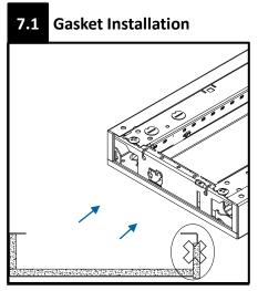
Ensure gasket is seated properly. Gasket should not protrude overall luminaire width and height.
