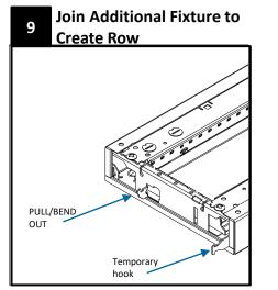
On the additional fixture, pull out the two tabs.
