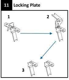
Brake locking plate in two halves
