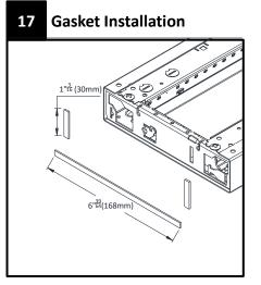
Cut, peel and stick gasket to edge of luminaire as shown. Refer to step 7-7.2 for more instructions.
