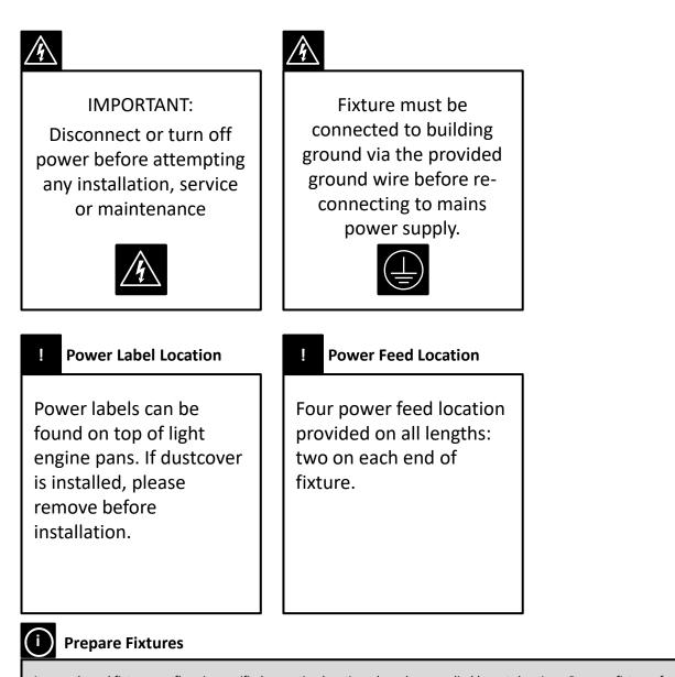
Arrange boxed fixtures on floor in specified mounting locations, based on supplied layout drawings. Remove fixtures from boxes **Note: If conditions are dusty/dirty, recommended practice is to leave fixtures in their plastic bags.**
