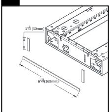
Cut, peel and stick gasket to edge of luminaire as shown. Every fixture end requires gasket installation.
