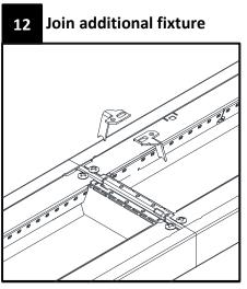
SLIDE MODULES TOGETHER: Drop in the locking plate provided in the joint kit. Locking plate will interlock the two fixtures together **3** Secure with locking plate
