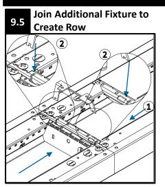
SLIDE MODULES TOGETHER UNTIL NO GAPS ARE VISIBLE: Drop in the locking plate provided in the joint kit. Locking plate will interlock the two fixtures together.
