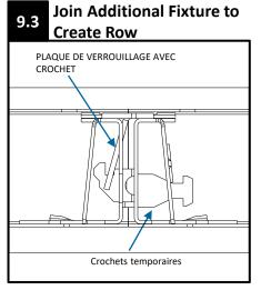
At joint, insert temporary hooks into suspended
