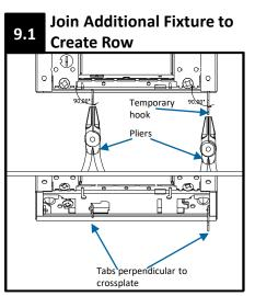
Using a set of pliers, ensure that tabs are perpendicular to fixture. This is required to ensure proper engagement to opposite fixture.
