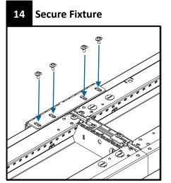
Fold wall mount bracket on top of joint fixtures. Using the provided Philips screws, lock the wall mount bracket to the fixtures
