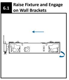
Once engaged on hooks, rotate fixture down into position.
