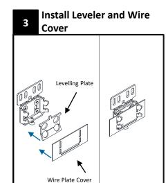
Place the levelling plate onto the bracket followed by the wire cover plate.
