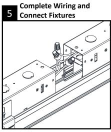
Install the joiner fixture into the T-Bar Grid from above. Complete wiring and slide the fixtures together.
