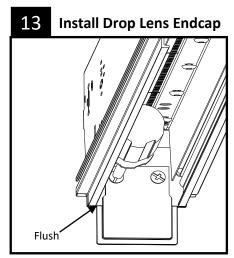
Push up drop lens endcap flush to bottom of trim while **hand tightening** with supplied screws.(8-18 x 3/8 Pan)
