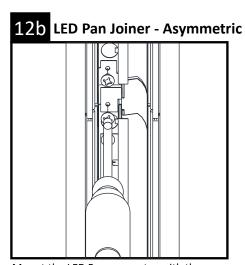
Mount the LED Pan connector with the supplied screw in the joiner kit. There are two pieces for asymmetric fixtures.
