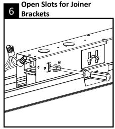
Snap off the safety cover on joiner brackets slots with a flat head screw driver. This only needs to be done one sides that require joining.
