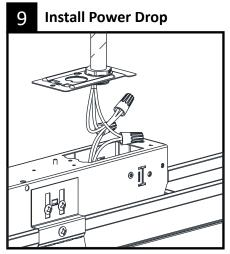
Install power drop at desired location. At power location(s), remove factory installed wire cover. Feed power wires through. Complete all wiring connections using wire nuts supplied by others.
