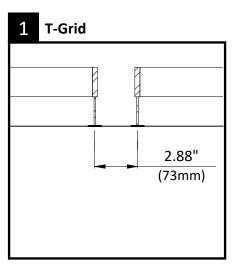
Install main tees, 2.88" on center. For continuous row lengths, refer to supplied layout drawings. Add 1/4" to the overall housing length indicated on your layout drawings. Position and secure the cross tees.
