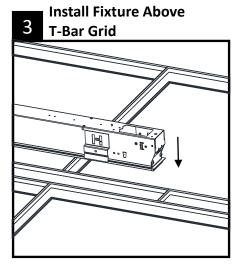
Install the first fixture (or Standalone Unit) from above the T-Bar Grid.
