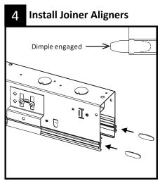
In the joining fixtures install the joiner aligners in the trim extrusion just past the halfway point.
