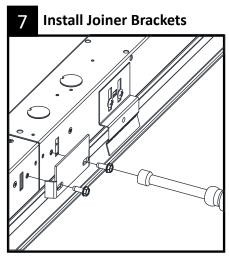
Install supplied joiner brackets with 5/16" nut driver.
