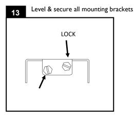
LEVEL: Using 5-16" nut driver, level fixture by adjusting the Tilt screw.
