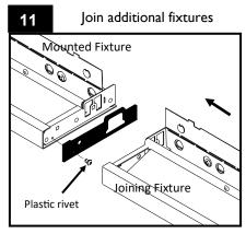
Insert the foam gasket onto the mounted fixture end. Using the supplied plastic rivet, fasten the gasket in place so it doesn't move during fixture joining.
