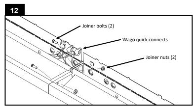
Ensure both fixtures are horizontal and mounted at the same height. Snug joining nuts using 3/8" nut driver, align the fixture housings for best aesthetic before final tightening. Complete necessary electrical connections in compliance with local codes. Close all wire access panels (step 9) when complete.
