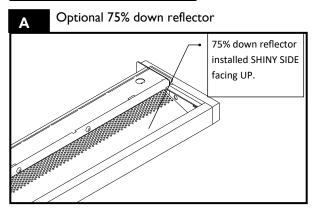
FloatPlane Fixtures available with a factory installed, perforated 75% down reflector. For best optical performance, reflector must be installed as shown, SHINY SIDE facing UP. Note down reflector is installed on top of clear acrylic upper diffuser.
