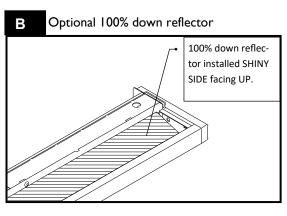
FloatPlane Fixtures available with a factory installed, solid 100% down reflector (shown as hatched lines). For best optical performance, reflector must be installed SHINY SIDE facing UP. Note down reflector is installed on top of clear acrylic upper diffuser.
