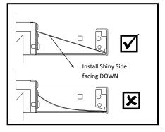
Re-install the upper diffuser (SHINY SIDE facing DOWN). If applicable, re-install optional 75 or 100% downlight reflectors on top of diffuser in correct orientation.
