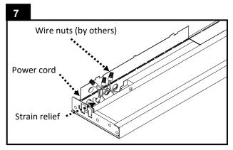
Crimp supplied strain relief onto power cord insulation (recommend Heyco Tool PN0019(R12). Complete necessary electrical connections (by others) in compliance with local codes. Push the wires and connectors back down into the wire compartment when complete.
