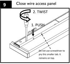
Ensure the electrical connectors are tucked inside the wire cavity. Push down on the lid while simultaneously twisting the flat blade screwdriver, the panel tab will lock into place. Repeat at the other screwdriver slot location.
