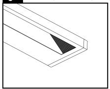
If the fixture is mis-handled during installation, a shadow may appear in the luminous window. This is caused by the upper diffuser being pushed below the LED.
