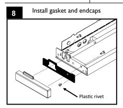
Insert the foam gasket onto the fixture end. Using the supplied plastic rivet, fasten the gasket in place so it doesn't move during endcap installation.
