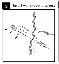
Install mount brackets to wall structure using appropriate fasteners (BY OTHERS). Note bottom of installed fixture will sit approx. 3/8" below bottom edge of bracket.
