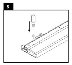
At power feed location on fixture. Insert a medium size flat blade screwdriver into slots on access panel.
