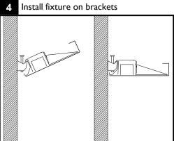
POWER LOCATIONS: Prior to engaging fixture on mounting brackets, feed installed power cord through one of the power access holes at the back of fixture.
