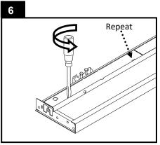
Twist the screwdriver and the tab on the access panel will POP UP. Repeat on the other tab on the access panel. Open the wire access panel.
