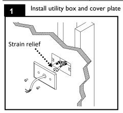
Determine power feed location and install 2"x4" utility box (supplied by others) parallel with fixture. Complete electrical connections at box with supplied power cord. Crimp supplied strain relief onto power cord insulation (recommend Heyco Tool PN0019(R12). Attach cover using supplied painted hardware.
