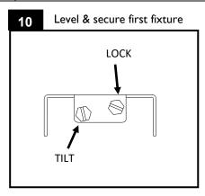
LEVEL: Using 5-16" nut driver, level fixture by adjusting the Tilt screw.
