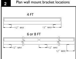
Determine wall mount bracket locations based on the allowable distance from fixture ends to brackets, and also factoring in site conditions (location of structural members).
