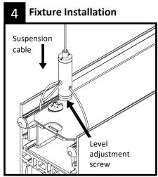
Raise fixture to installed level and insert suspension cable inside sling cable assembly. Ensure end of aircraft cable exits from sling cable assembly as shown.
