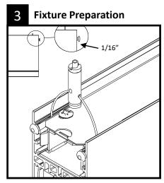
Attach two push pins to screw chases to secure sling cable assembly inside fixture during installation process. Gently tap each push pin into the housing leaving a 1/16" gap for easier removal later.
