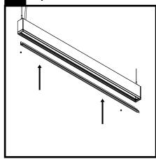
Reinstall the lower led pans with the screws provided. Ensure direction of light is as shown on layout drawings.
