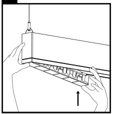
Installation Tip: For easier installation, start on one end of the louver pressing gently on side tabs. **IMPORTANT:** For asymmetric louver fixtures, orientate the arrows on the louver pan to point at the label on the outside of the housing.
