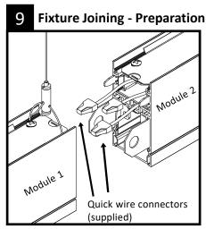
Raise module 2 to installed module 1 position. Install and secure sling cable assembly of module 2 and at opposite. Remove push pins from module 1.
