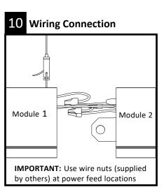
Bring modules close together, support module 2, complete wiring connections and tuck wires inside fixture wiring cavity. Engage joiner aligners from module 2 inside module 1.
