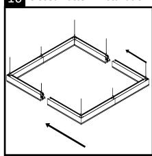
If installing a square or rectangular closed pattern, it is recommended to install opposite U-shaped fixture/corner patterns first and complete the installation by bringing U-shaped sections together as shown.
