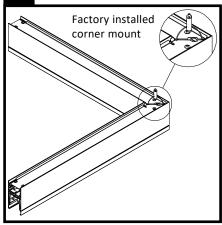
If a corner is required, it is recommended the corner module be installed first. All corners come with a factory installed cable sling assembly in the middle.
