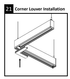
Installation filler plate before installing louvers. Tip: For easier installation, start by squeezing filler plate in slightly from both sides and guiding inside housing.
