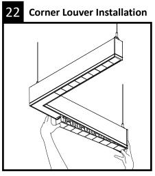
Installation Tip: For easier installation, start on one end of the louver pressing gently on side tabs.
