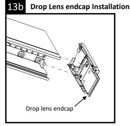
Place drop lens endcap as shown over the emboss of endcap and proceed with endcap Installation of endcap, step 14.
