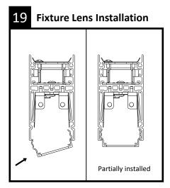
Install lenses removed in step 1. Installation Tip: For easier installation, start at a housing end or a joint by placing lens at an angle and squeezing in slightly from the other side to guide inside housing.
