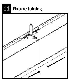
Ensure all connections are secure and all wires are fully tucked inside fixture wiring cavity. Slide fixture modules together gently. Level fixtures.
