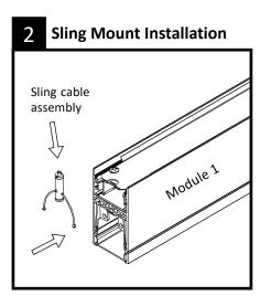
With module 1 on the ground, slide sling cable assembly into top fixture screw chase on both ends of the fixture.
