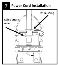
Install and crimp provided cable metal strain relief bushing to secure power cord below fixture reflector. Use a Heyco PN0019(R12) crimping tool to ensure proper installation. If installing a standalone fixture, **skip to step 13**.
