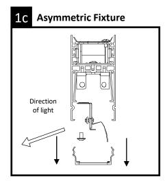
Remove lens and set aside until fixture installation is complete. Use cotton gloves to handle lenses and keep in a clean environment.
