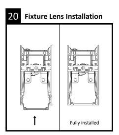
Once lens is positioned inside housing, starting on one end or joint, push upwards gently and work outward to complete the
