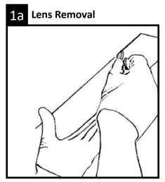
Lens Removal: To remove snap-in lens for maintenance purposes, insert a flat, smooth edged object between lens and housing (avoid screwdrivers). Twist to release pressure and remove lens.
