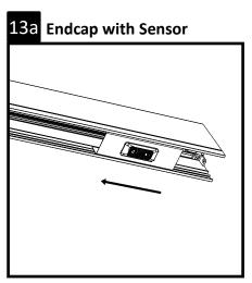
Before installing the endcap, slide the sensor towards the center of the fixture to gain access. Proceed with endcap installation, step 14.
