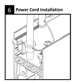
Determine power feed location and break ½" electrical knockout at required end. Install ½" bushing from above fixture as shown. Feed power cord from above into fixture wiring cavity.
