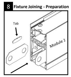
With module 2 on the ground, tap small joiner aligners inside top screw chase. Insert larger joiner aligners inside lower screw chase as shown.
