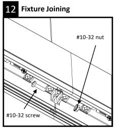
Secure fixture modules together using the two #10-32 machine screws and the two self-locking #10-32 nuts supplied. Tighten until joint seam is tight.
