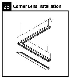
Installation Tip: For easier installation of corner lenses, start at the corner and work outward to complete the run. Follow steps 19 and 20.
