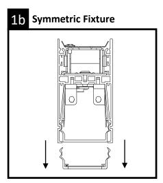
Remove lens from fixture and set aside until fixture installation is complete. Use cotton gloves to handle lenses and keep in a clean environment.
