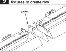
With two people, raise second fixture and engage on mounting brackets (see STEP 4). At joint, remember to insert black gasket.
