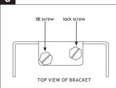
LEVEL: Using 5/16" hex nut driver, level fixture by adjusting the tilt screw.
