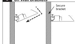
With 2 people, raise fixture into position and engage it on hooks located on top of wall brackets, then rotate it down into position. Secure bracket using supplied hardware.
