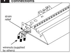
Complete electrical connections using wire nuts (supplied by others). Re-install pan and hardware removed in STEP 5.
