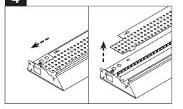
Shift top reflector to the left and then remove the reflector.
