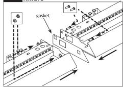
Level second fixture by adjusting the tiltscrew (see step 8). Slide second fixture flush against first fixture and secure joint using supplied nut and bolt hardware (requires 3/8 nut drivers). Secure fixture to wall brackets by tightening the lock screw at each bracket location (see step 8).
