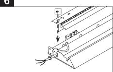
To access wiring, remove screw from top pan and lift pan off. Apply strain relief to power cord.
