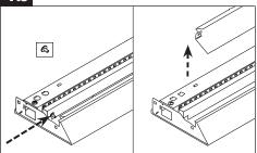
Remove the screws holding the front reflector and then remove the front reflector.
