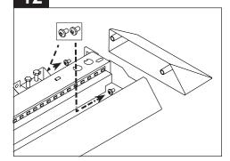
Attach endcap to first and last module in each row using supplied hardware.
