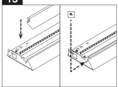
Re-install front reflector using short (stubby) screwdriver.
