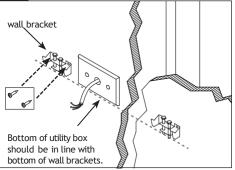
Determine fixture mounting location and secure wall brackets to structure using appropriate fasteners (two per bracket, supplied by others). 4ft fixtures: Require two bracket assemblies; 8ft fixtures: Require three bracket assemblies. Brackets must be installed a maximum of 5" from end of fixture (on 8ft fixture, the third bracket can be 5" of ether side of inrow crossplate).
