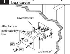
Determine power feed location and install 2"x4" utility box (supplied by others) parallel with fixture. Complete connections at utility box with supplied power cord. Attach cover bracket using supplied hardware. Punch power access hole in supplied cover, feed power cord through and attach strain relief on wall side. Attach cover using supplied painted hardware. NOTE: Bottom of utility box should be in line with bottom of wall brackets.
