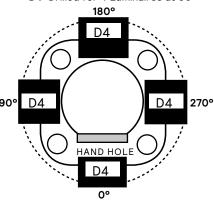
D2@90 Drilled for 2 Luminaires at 90°
