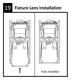
Once lens is positioned inside housing, starting on one end or joint, push upwards gently and work outward to complete the run.
