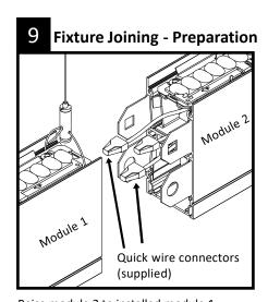
Raise module 2 to installed module 1 position. Install and secure sling cable assembly of module 2 and at opposite. Remove push pins from module 1. **IMPORTANT: WIRING INSTRUCTIONS** Quick wire connectors (supplied) are used for through wiring connections between fixtures. Wire nuts (by others) are used for connection of power drops wiring to fixture
