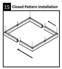
If installing a square or rectangular closed pattern, it is recommended to install opposite U-shaped fixture/corner patterns first and complete the installation by bringing U-shaped sections together as shown.
