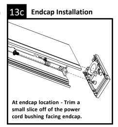
Slide endcap onto end of fixture module and secure from below using two #8-32 X 3/8" screws. Ensure excess aircraft cable does not interfere with endcap attachment. Use ratchet or angle driver to tighten screws until endcap seam is tight.
