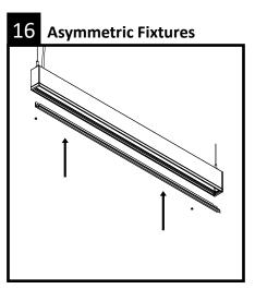
Reinstall the lower led pans with the screws provided. Ensure direction of light is as shown on layout drawings.
