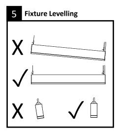
Ensure module 1 is installed level. Do not install at an angle.
