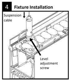
Raise fixture to installed level and insert suspension cable inside sling cable assembly. Ensure end of aircraft cable exits from side of sling cable assembly as shown.
