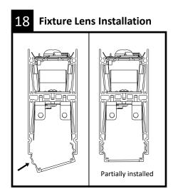
Install lenses removed in step 1.
