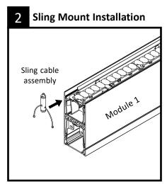
With module 1 on the ground, slide sling cable assembly into top fixture screw chase on both ends of the fixture.
