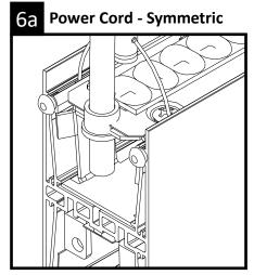
Determine power feed location and break ½" electrical knockout at required end. Install ½" bushing from below fixture as shown. Feed power cord from above into fixture wiring cavity.
