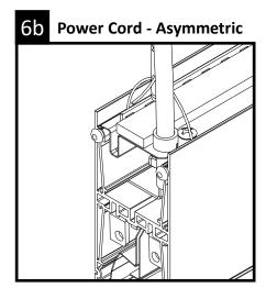
Determine power feed location and break ½" electrical knockout at required end. Install ½" bushing from inside fixture as shown. Feed power cord from above into fixture wiring cavity.
