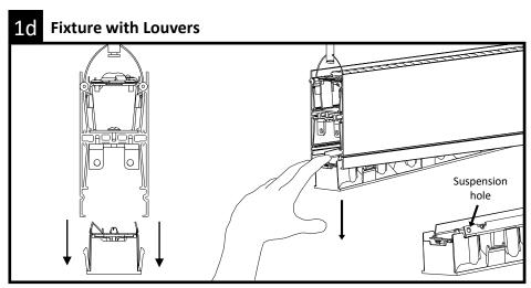
Remove one louver from end of fixture by pulling gently and temporarily suspend from available holes.
