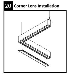
Installation Tip: For easier installation of corner lenses, start at the corner and work outward to complete the run. Follow steps 18 and 19.
