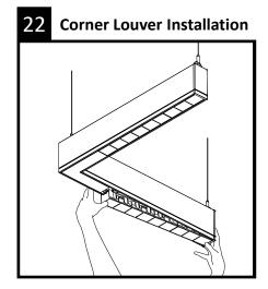
Installation Tip: For easier installation, start on one end of the louver pressing gently on side tabs.
