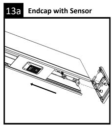
Before installing the endcap, slide the sensor towards the center of the fixture to gain access. Proceed with endcap installation for drop lens, step 13c.
