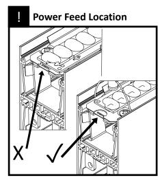
If installing a fixture with one power feed location, ensure electrical knockout orientation matches required power feed location.
