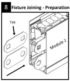
With module 2 on the ground, tap joiner aligners inside top and bottom screw chases as shown.
