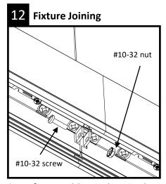
Secure fixture modules together using the two #10-32 machine screws and the two Self-locking #10-32 nuts supplied. Tighten until joint seam is tight.
