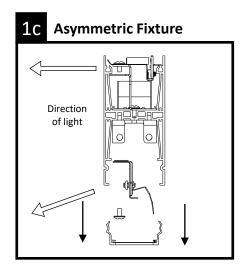
Remove lens and set aside until fixture installation is complete. Use cotton gloves to handle lenses and keep in a clean environment.
