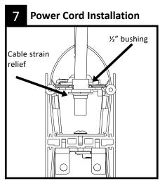
Install and crimp provided cable metal strain relief bushing to secure power cord below fixture bracket. Use a Heyco PN0019(R12) crimping tool to ensure proper installation. If installing a standalone fixture, skip to step 13.
