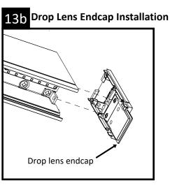
Place drop lens endcap as shown over the emboss of endcap and proceed with endcap Installation of endcap, step 13c.
