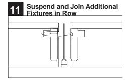
Raise next fixture to cantilever bracket and insert the joiner aligners into the corresponding slots on the already installed fixture.
