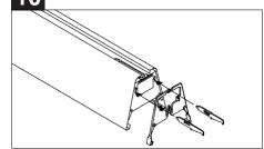
On the floor, slide variable mount bracket into next fixture in run. Attach joiner-aligner brackets into opposite side.
