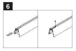
On the floor, slide power plates into fixture ends. Attach supplied bushings in power locations and plugs in non-power locations.
