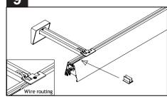
Run power cable in fixture channel and through power plate at the end of the fixture. Secure power cable into fixture channel using supplied cable clips at 4 increments.
