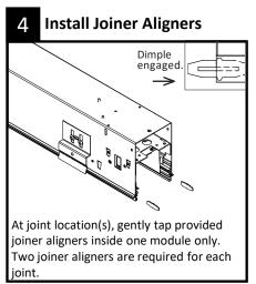
Important: To insert aligners, tap gently with a hammer until half is inserted into the joiner channel. Be sure to engage the dimple. 5 Complete Wiring and Connect Fixtures
