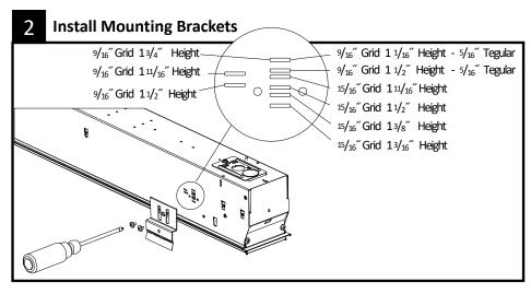
Important: Install T-Grid mounting brackets to required height.
