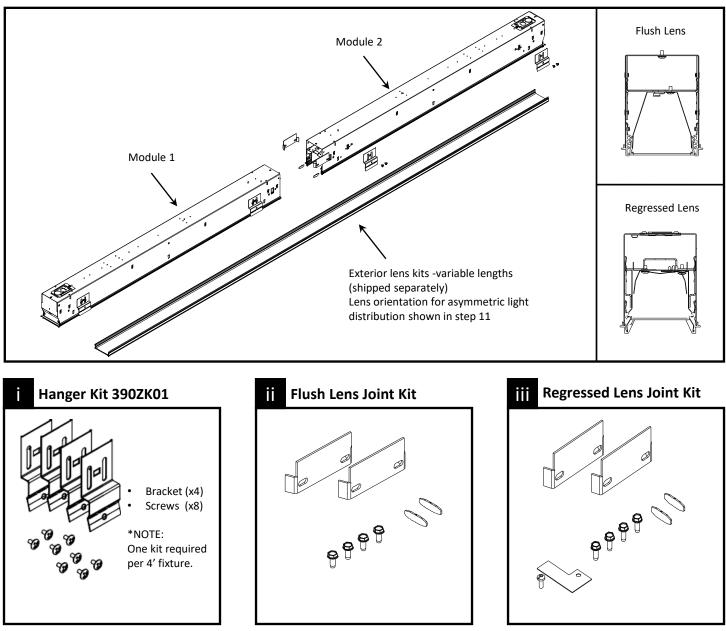
\*Note: One kit required for each joint. Joint kit type determined by flush or regressed lens. Tools: Phillips screwdriver, 5/16" Nut Driver
