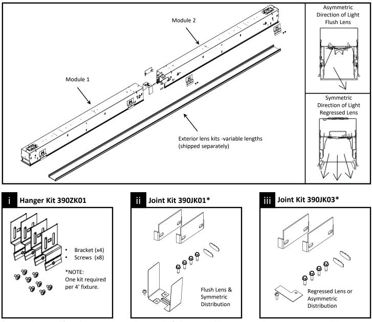
\*Note: One kit required for each joint. Joint kit type determined by flush or regressed lens mounting and symmetric or asymmetric light distribution. Tools: Phillips screwdriver, 5/16" Nut Driver
