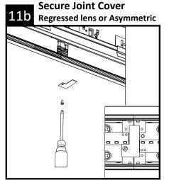
At joint location(s), secure joint covers using Philips screwdriver and supplied hardware. Ensure cover plates sit flush with bottom reflectors for proper LED board fit.
