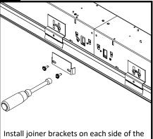
Install joiner brackets on each side of the housing using supplied hardware.
