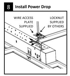
Install power drop at desired location. At the power location(s), remove factory installed wire cover. Feed power wires through. Complete all wiring connections.
