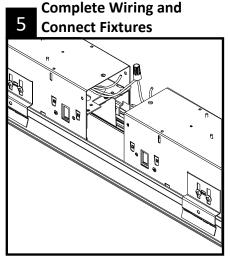
Install the joiner fixture into the T-Bar Grid from above. Complete wiring and slide the fixtures together. 6 Install Joiner Brackets
