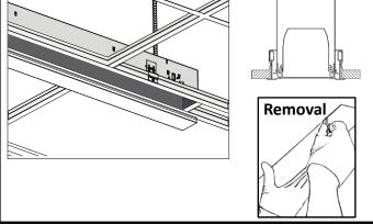
Flush Lens: Snap in lens into fixture.
