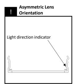
Note the knob on the inside of the lens. The asymmetric film directs to light in the direction of the knob. Always install in the fixture in the direction shown on the layout drawings.
