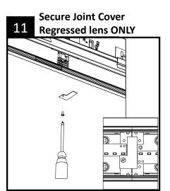
At joint location(s), secure joint covers using Philips screwdriver and supplied hardware. Ensure cover plates sit flush with bottom reflectors for proper LED board fit.
