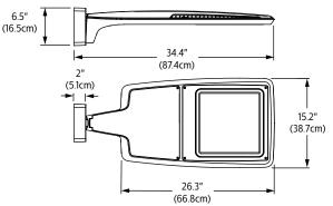
Slip fitter (SF) Weight: 32 Lbs (14.6 Kg) EPA: 0.38ft<sup>2</sup> (.035m<sup>2</sup>)
