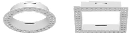
**Mud-in ring (WH):** Low profile, machined aluminum mud-in ring provides a raised rib to plaster up to and a 3/16" flange thickness. The ring is attached to the ceiling material directly via flat head screws (contractor supplied).
