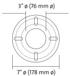
Bolt circle 5-1/2" (140mm) B.C. possible: from 4-3/8" to 6" (111mm to 152mm)
