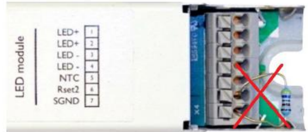
Example of improper use of a non-isolated Rset2 resistor; the bottom lead wire is positioned too close to the driver housing. Contact with the metal driver housing may result in driver malfunctioning or failure.
