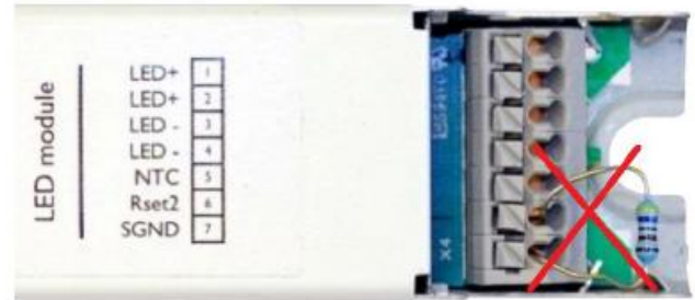
Example of improper use of a non-insulated Rset2 resistor; the bottom lead wire is positioned too close to the driver housing. Contact with the metal driver housing may result in driver malfunctioning or failure.
