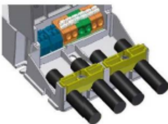
Strain relief blocks for the WH driver for independent application. Screws must be fastened with 0.8 ... 1.2Nm torque. The cable clamp supports cable diameters between 6 ... 10mm.
