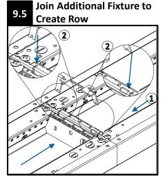
SLIDE MODULES TOGETHER UNTIL NO GAPS ARE VISIBLE: Drop in the locking plate provided in the joint kit. Locking plate will interlock the two fixtures together.
