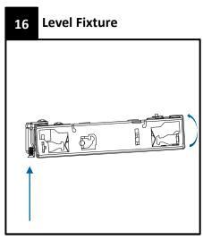
Level fixture using the 8-32 x ½" screw with a screwdriver.
