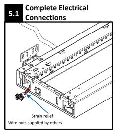
NON-POWER LOCATIONS: Cap all wires and tuck into wire cavity. POWER LOCATIONS:
