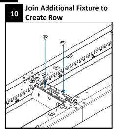
Once locking plate is inserted, secure locking plate to the crossplate. Using a head screwdriver, tightened screws until the two fixtures pull together creating a seamless gap.
