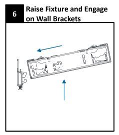
With two people, raise fixture into position and engage it on hooks located on top of wall brackets.
