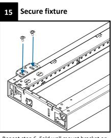
. Repeat step 6. Fold wall mount bracket on top of fixture. Using the provided Philips screws, lock the wall mount bracket to the fixtures
