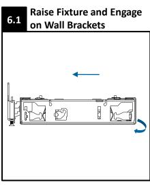
Once engaged on hooks, rotate fixture down into position.
