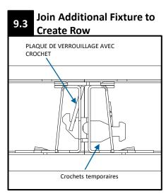
At joint, insert temporary hooks into suspended
