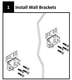
Determine fixture mounting location and secure wall brackets to structure using appropriate fasteners (four per bracket, supplied by others). 4ft fixtures: Require two bracket assemblies; 6ft & 8ft fixtures: Require three bracket assemblies. Brackets must be installed a maximum of 1.6" from end of fixture (on 6ft & 8ft fixture, the third bracket should be installed in the middle). See page 2 for mounting bracket location.
