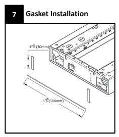
Cut, peel and stick gasket to edge of luminaire as shown. Every fixture end requires gasket installation.
