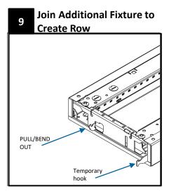
On the additional fixture, pull out the two tabs.
