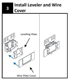
Place the levelling plate onto the bracket followed by the wire cover plate.
