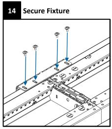
Fold wall mount bracket on top of joint fixtures. Using the provided Philips screws, lock the wall mount bracket to the fixtures
