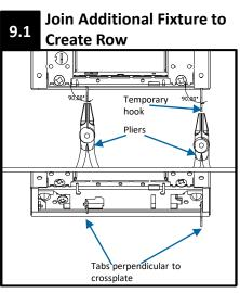
Using a set of pliers, ensure that tabs are perpendicular to fixture. This is required to ensure proper engagement to opposite fixture.
