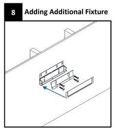
In the event of a row, the mid run bracket needs to be installed instead of the end of run bracket. See page 2 for more details.
