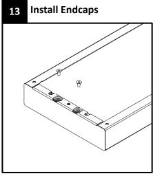
Using the provide Phillips screws (black), attach endcaps to bracket.
