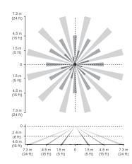
**Note:** The beam patterns shown are intended solely as a general guide and are not to scale. Sensing capabilities and coverage area depend on many factors including the size, speed and direction of travel of persons and vehicles; sensor mounting height; environmental and site conditions; etc.
