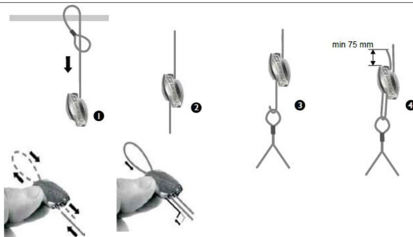
It is required to use special Grapple suspension set No. 3 with different then express fastener system
