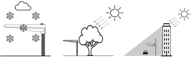
The luminaire performance and battery charging can be affected by external parameters.
