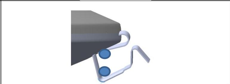
MAKE NECESSARY ADJUSTMENTS TO THE CLIPS AND WIRE GUARD TO ENSURE A PROPER FIT. SCREW UPPER LENS TO LOWER CASTING AND INSTALL FIXTURE.
