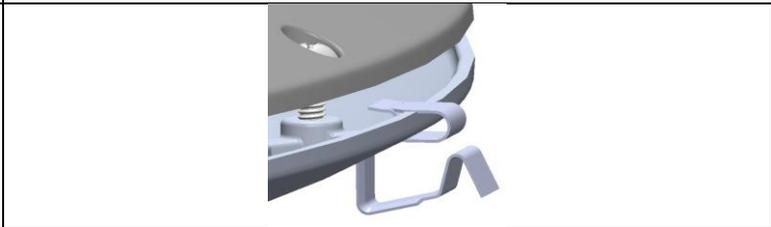
MOUNT THE WIRE GUARD TO THE FIRST CLIP UNDER THE TOP TWO RINGS. USE NEEDLE NOSE PLIERS TO SPREAD THE CLIP. BE SURE TO WEAR GLOVES WHEN HANDLING THE CLIP.
