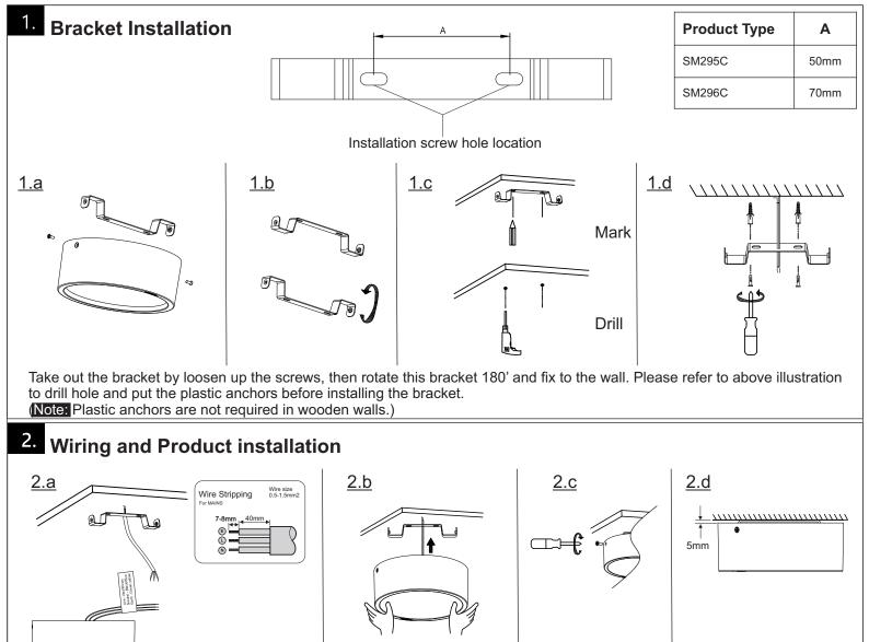
Connect the mains wires to L-N-E wires of the product. (Note: Turn off the power before installation). Align the product with mounting bracket and screw from 2 sides. please refer to above illustration. There will be 5mm gap between product and ceiling after mounting.
