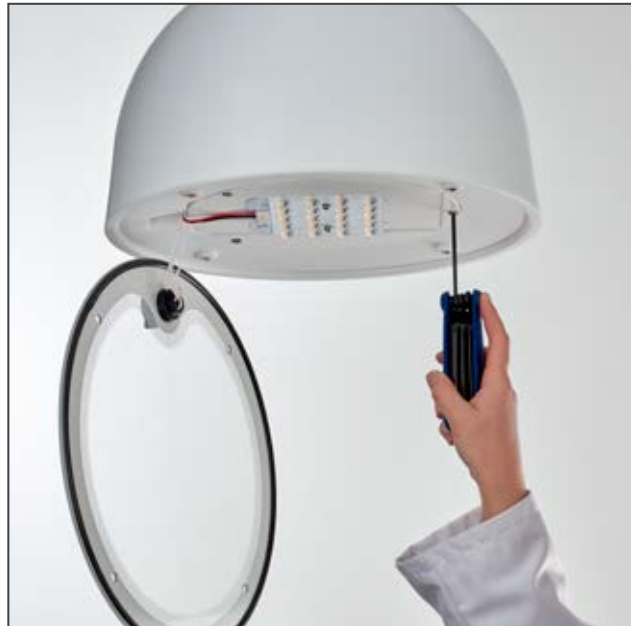
Untight two screws of the mask and remove it.
