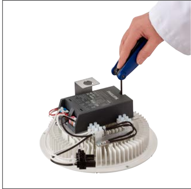
Unscrew two screws to remove the driver. Install the new driver. Loosen two screws and remove LED board.
