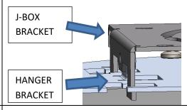
REPLACE THE SET SCREW LOCATED AT THE FRONT OF THE TOP SHEET METAL BRACKET. TORQUE TO 19 IN. LB.
