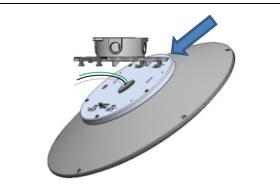
PUSH THE FIXTURE UP LEVEL SO THAT THE JUNCTION BRACKET ENGAGES WITH THE FRONT HANGER BRACKET.
