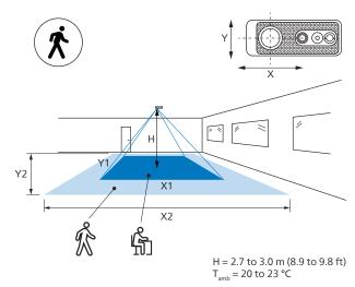
The detection area is sensed by a single pixel thermopile. By software processing the information is processed to radiant temperature at surface level.
