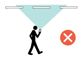
Holding the phone closer to eye level or lower will result in a wider IR range or cone. This will cause multiple luminaires to receive the signal.
