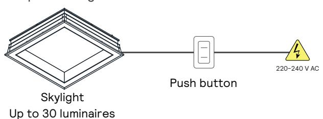
When the light is turned on via the push button (short push), the driver will recall the last dim level.
