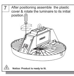
Rotate the luminarie so that plastic cover towards the installer for ease of installation/ maintenance. Remove the plastic cover by open 2 screws with screw-driver.
