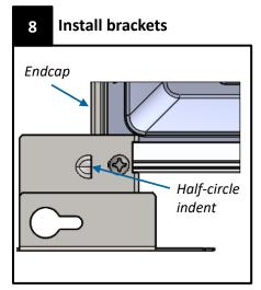
The bracket <u>MUST</u> fully rest on the aluminum extrusion, and the endcap <u>MUST</u> be touching the flat side of the Half Circle Indent on the bracket. Install a bracket at each corner with one 8-18 Phillips/Robertson pan head screw provided (*DO NOT overtighten*). Repeat for all four corners.
