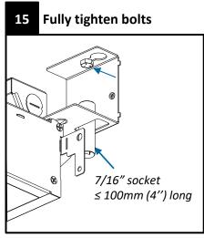
Slide fixture to the narrow end of the key holes. Fully tighten bolts. Use 7/16'' socket x 3/8 sq drive with extension with minimum total length 100mm (4.0"). For studs, install washers and nuts and fully tighten.
