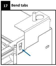
Push down the tabs over the bracket, about 120 degrees. The tabs prevent the box from falling during installation.
