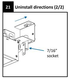
Loosen hex head bolts with 7/16" socket with extension.
