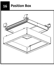
Lift box up around the suspended fixture with brackets. Tabs will prevent the box from reaching the ceiling.
