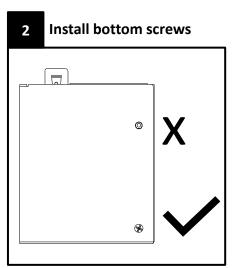
Arrange panels into a box. Install 4x 8-18 Phillips white painted screws at the bottom corners. Do not install top screws. Check that corners are tightly joined.
