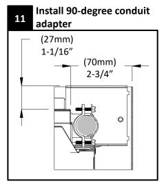
A 90-degree elbow, 3/4 female x 3/4 NPSM male conduit adapter is recommended. Clearance between driver box and cover is 2.75" (70mm). Clearance from the top of the standard driver box to ceiling is 1-1/16" (27mm). For the Emergency Driver box, the clearance to the ceiling is 3/8" (10mm).
