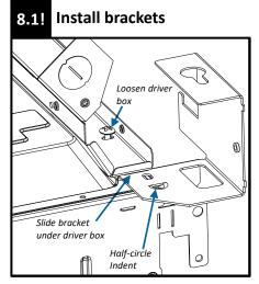
If the driver box prevents the Half-circle indent from touching the endcap, slightly loosen the screws fixing the driver box to the aluminum extrusion and slide the bracket underneath without unhooking the wiring. Lastly, retighten the driver box's screws and close it.
