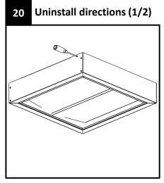
To uninstall the surface mount frame and service the driver box, remove 4 screws from top of the box and lower the box. Unbend tabs at each corner and remove panels. NOTE: Two people are recommended for this step and following steps for 1'x4' and 2'x4' fixtures.
