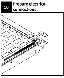
Prepare electrical conduit connections to the driver box. See installation sheet for electrical connections instructions for Duo Recessed Families - Installation Sheet: *IS-Duo* (steps 5-7).
