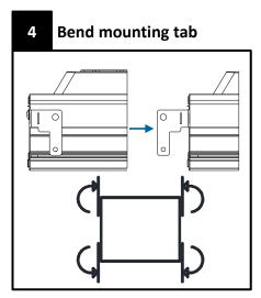
Place the lighting fixture on a flat surface. The mounting tab will be bent close to the aluminum extrusion on the 4 corners.
