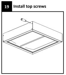
Lift the box to have the bracket holes in line with the box top holes. Install 4x 8-18 Phillips white painted screws at the top corners, through the end panels to the brackets. Use #2 Phillips screwdriver. Installation is complete.
