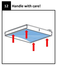
NOTE: DO NOT PUSH ON FIXTURE LENS! ONLY SUPPORT FIXTURE BY SIDE ALUMINUM RAILS.
