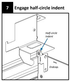
Rotate the bracket onto the extrusion. Adjust the position of the bracket until the half circle indent is touching the endcap. NOTE: Follow steps 8 and 8.1 closely to ensure proper engagement.
