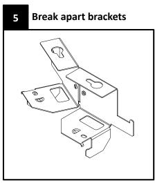
Bend brackets back and forth to weaken connector tabs and snap apart into two pieces. Repeat for second bracket. You will now have four pieces.
