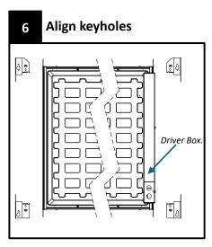
Place one bracket beside each corner. Align keyholes to each other. Keyholes are oriented parallel to the driver box.
