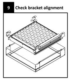
Dry fit the fixture with brackets into the assembled box (do not install top screws). Check bracket hole alignment with the holes in the box. The fixture will sit approximately 1mm above the bottom of the box. Remove fixture from assembled box.
