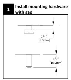
Install four  $\frac{1}{3}$ " hex head bolts or  $\frac{1}{3}$ " studs (supplied by others) in locations Mount X and Mount Y according to table above. Do not fully tighten. For bolts: leave a 6mm (1/4") gap to the ceiling. For studs: leave a minimum 16mm (5/8") gap to ceiling.
