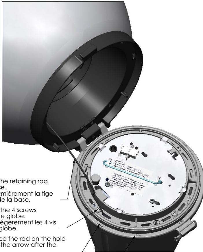
First detach the retaining rod from the base.
