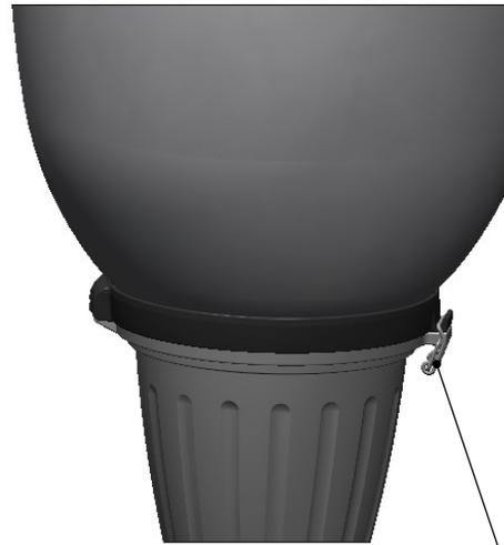
For maintenance, pull the locking device and then open the globe.
