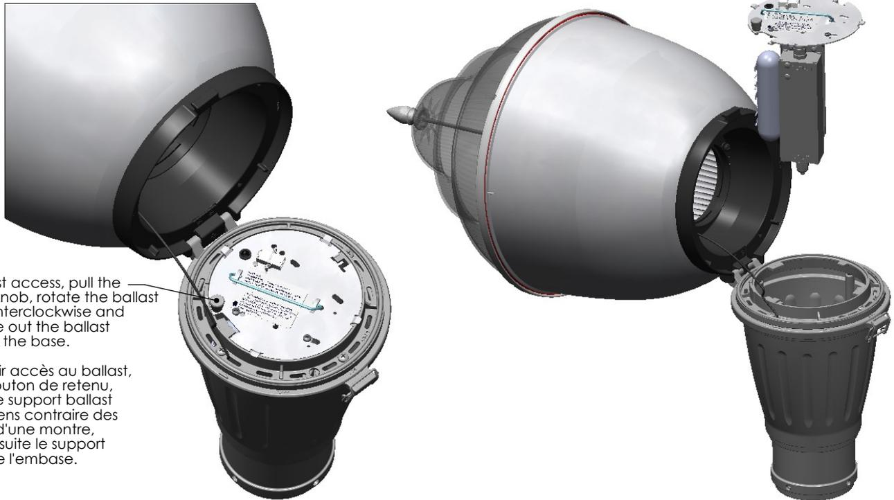
For ballast access, pull the security knob, rotate the ballast tray counterclockwise and then take out the ballast tray from the base.
