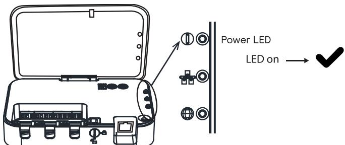
Test the connection with the luminaires by pressing the service button
