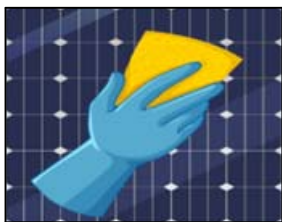
Use gloves to clean PV panel
