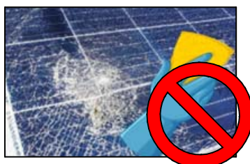
Do not clean broken PV panel
