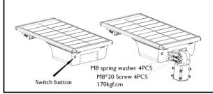
Step 3: Loosen the screws on the universal support and adjust the irradiation Angle of the solar panel. Tighten the screws with a torque of 600kGF. cm and adjust the Angle of  $-90^*$ -+90. It is recommended that the installation Angle be 15 degrees (preparation tool :14MM hex wrench).
