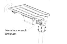
Step 2: A: Put the lamp into the pole, tighten the M10 screw with a torque of 250kGF. cm. B: tighten the M10 nut with a torque of 150kGF. cm (preparation tools:5MM inner hexagon wrench,17mm outer hexagon wrench)
