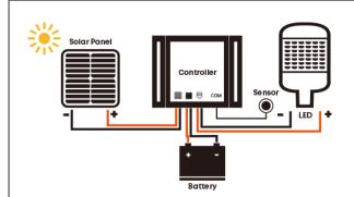
During the day, the solar light shines on the solar panel, generating electric energy, which is controlled by the controller to charge the battery. In the evening, the solar light darkens, the controller stops charging, and then drives the LED light to turn on. If there is an induction function, the light becomes bright when the induction, and the light becomes dark when there is no induction.
