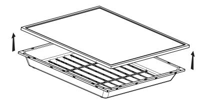
Open Snap Locks from Diffuser Frame to open the Fitting for access.
