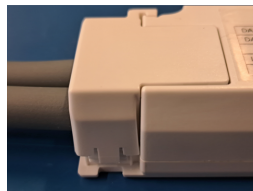
Correct placement strain relief cap
