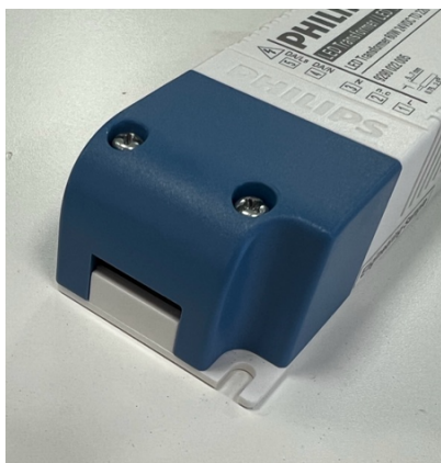
Strain Relief Cap Screws must be fastened with 0.5N.m torque. The input cable clamp supports cable diameters between 3.5 ... 8mm. The output cable clamp supports cable diameters between 3 ... 8mm.
