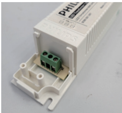
Connectors Recommend torque for screws is 0.3N.m
