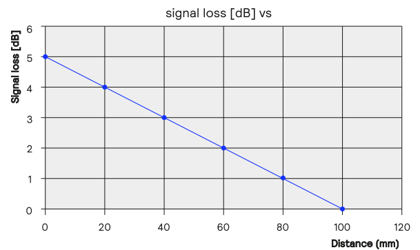
Transmission signal loss [dB] with distance to metal side wall [mm]. Closer the metal wall, higher the signal loss.
