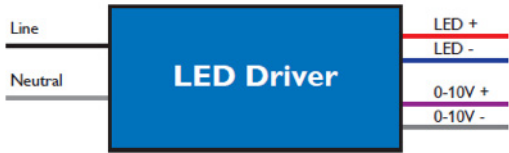
Figure 6. LED driver with 0–10V dimming interface
