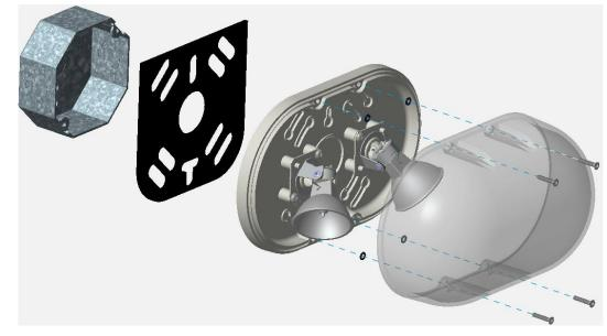
Remove the clear front cover by loosening the four screws that attach it to the mounting plate (Screws are retained by O-rings. Screws do not have to be removed from the clear cover, just the mounting plate.) Remove desired knockouts from mounting plate, applied supplied gasket and secure to junction box or mounting surface. Replace front cover.
