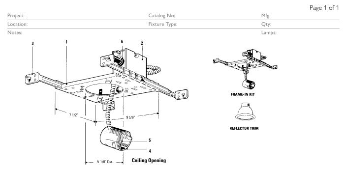
Complete Fixture consists of Reflector Trim & Frame-In Kit. Select each separately.
