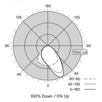
Definition Symmetric Flush Silk Lens - LN Spacing Criteria: 1.23/1.21
