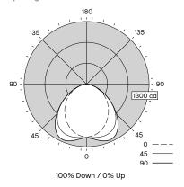
Performance Asymmetric Flush MesoOptic Lens - WN Spacing Criteria: 1.66/1.34
