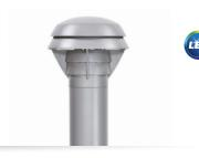
Gardco LED round full cutoff bollards feature LEDs concealed below cast louvers to provide down lighting for landscape and pathway applications. The BR40 series bollards have 4" diameter extruded aluminum shafts. Available mountings include the standard shaft, with a welded cast base mounted firmly to anchor bolts. They are also available with a galvanized steel base tenon reinforced shaft (BR842) for applications requiring additional support, such as schools.
